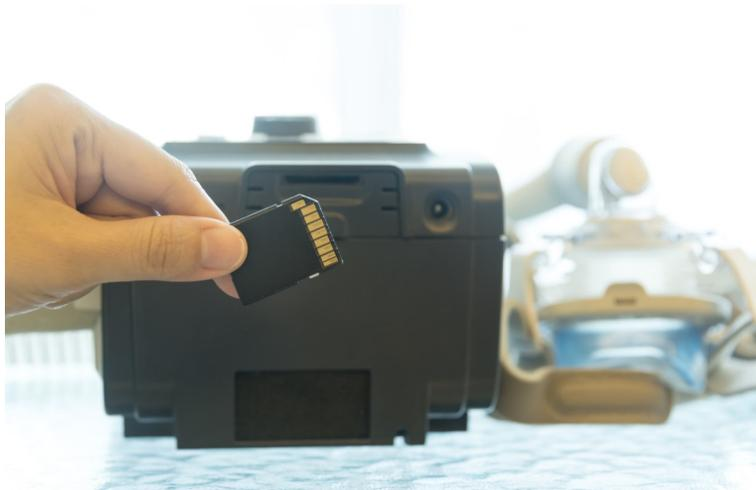
**Smart Card/Data Card:** A smart card or a data card is a memory storage device that works with PAP devices. The card should be in your PAP device, and you should bring it with you to each provider visit. The data card is then downloaded during your office visit. The data card conveys essential data to your provider, including frequency and duration of PAP device use, mask leak and residual apnea frequency.
